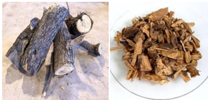
Figure 5: Sample 202348/5 – Olive trunks before and after chipping
