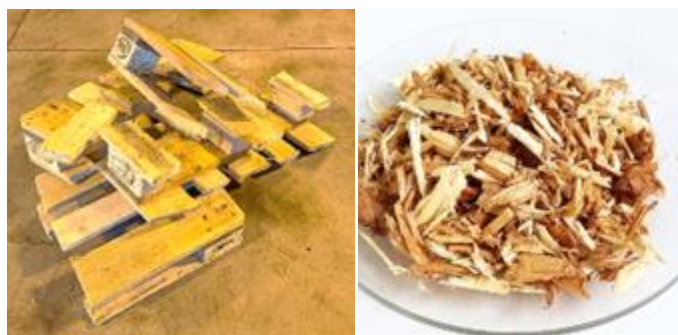
Figure 1: Sample 202348/1 – Pallet wood before and after chipping
