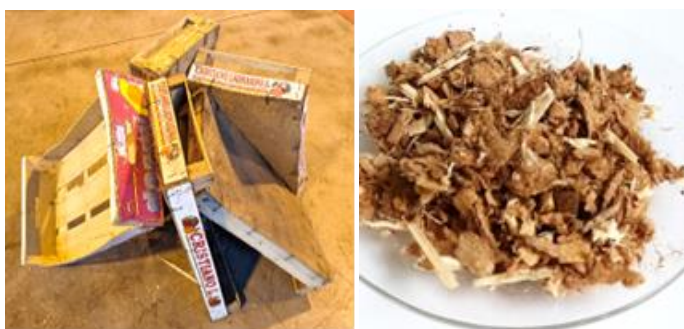
Figure 7: Sample 202348/7 – Boxes with chipboard bottom before and after chipping
