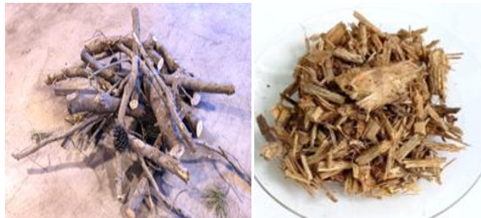
Figure 2: Sample 202348/2 – Pine wood before and after chipping
