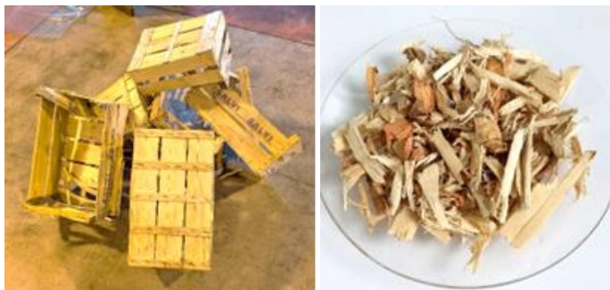
Figure 6: Sample 202348/6 – Boxes with plywood bottom before and after chipping
