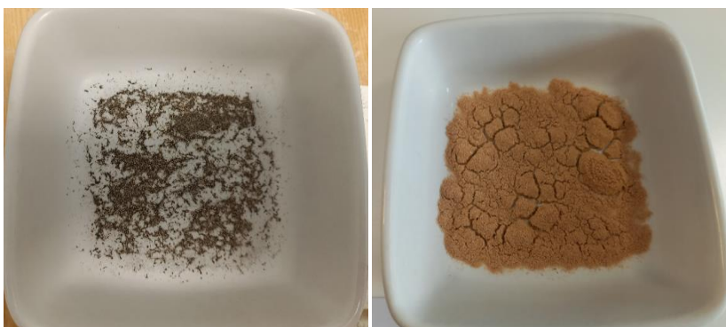
Figure 13: Ashes from straw (left) and coal (right) obtained from the same initial quantity of material
